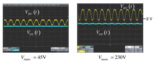
Figure 10. As Long as the Mains is Present, The  $V_{GS}$  Voltage of  $Q_2$  is Kept Low Enough to Block It
