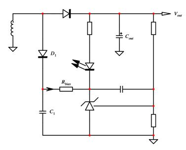
Figure 2. The Voltage across C<sub>1</sub> Collapses in Skip Cycle and the Bias Disappears on the TL431
