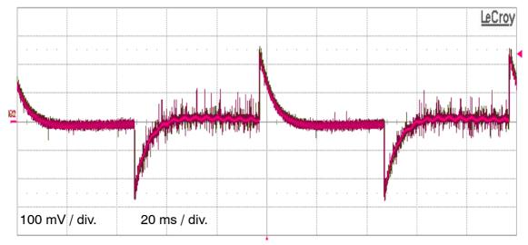
Figure 3. The Bias Suppression Circuitry Does Not Affect the Transient Response of the Adapter
