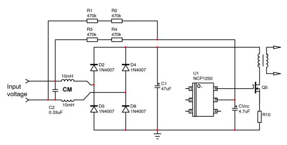
Figure 13. By Joining the X2 Resistors Terminals to the NCP1250 VCC Pin, it Naturally Combines the Discharge and Start-up Functions
