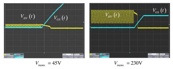
Figure 11. When the Mains Disappears, the Voltage on Q2 Gate–Source Terminals Quickly Rises Up and Triggers the X2 Capacitor Discharge
