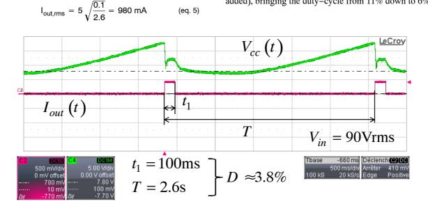
Figure 8. A Simple Bipolar Transistor Can Do the Job of Extending the Controller Off-Mode Period
